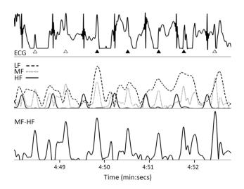
Fig. 3 – QRS detection, patient with pacemaker. Top: raw, damaged ECG. Middle: Frequency envelopes. Bottom: subtraction MF – HF, preventing detector from raising false QRS complexes by pacemaker stimuli. Detected QRS are shown at the top as white and black triangles, although in the case of a seriously damaged signal the distinction between regular and ventricular beats is not reliable (record "v5851").
