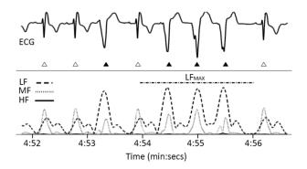
Fig. 2 – QRS detection. Top: raw ECG signal with detected QRS. White triangles are regular beats – Group 1, black triangles are ventricular beats – Group 2. Bottom: three amplitude envelopes for frequencies 1–8 Hz (LF), 5–25 Hz (MF) and 50–70 Hz (HF). The  $LF_{MAX}$  line marks the area with non-interrupted LF dominancy (record "v532s").
