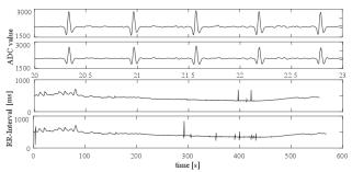
Figure 5. Results of treadmill exercise. Starting from the top: ECG (silicone electrodes); ECG (adhesive electrodes); RR-intervals (silicon electrodes); RR-intervals (adhesive Ag/AgCl electrodes)
