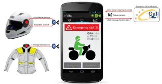
Figure 1. System overview: Electronics in helmet and garment are connected via Bluetooth. App can be notified by electronics to trigger eCall compliant emergency message.
