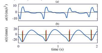
Figure 3. Example of the BPF method. Once the displacement is computed, the depth of each compression is estimated (red lines) and compared with the reference depth (green lines).
