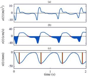
Figure 4. Example of the ZCV method. Once the velocity is computed, the depth of each compression is estimated and compared with the reference depth.
