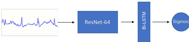
Figure 1: Deep learning model structure of ResNet+BiLSTM. ResNet is used to extract complex features from the ECG time series, and BiLSTM is used to build a prediction model based on the temporal order of features.
