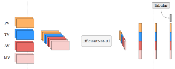
Figure 1. The model takes as input crops of mel-spectrograms of up to four different auscultation locations (PV, TV, AV, MV). The crops are reshaped and forwarded into a feature extractor. A reshape and pool operation pools multiple crops from the same time-series of the same valve. The four resulting pooled embedding vectors are concatenated with each other and with tabular features, and fed into a stack of linear layers for the competition tasks (not shown here).
