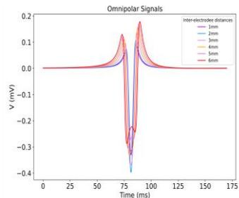
Figure 1. Omnipolar signals collected from inter-electrode distance between 1mm and 6mm.
