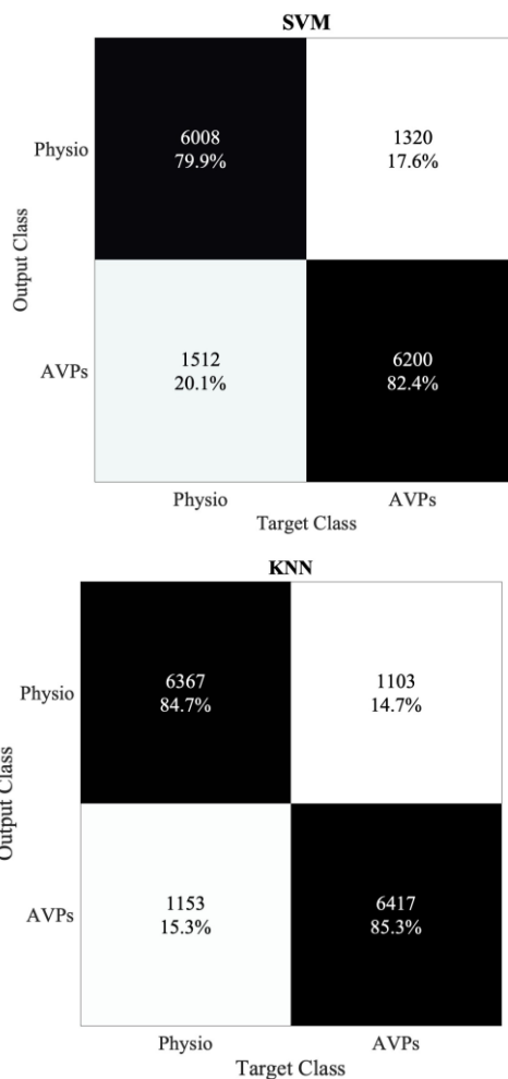
Figure 3. Cumulative confusion matrices for the two classifiers. In each matrix, the TPR (black box on the bottom-right corner) and the TNR (black box on the top-left corner) are reported along with their respective false negative rate (white box on the top-right corner) and FPR (light box on the bottom-left corner).
