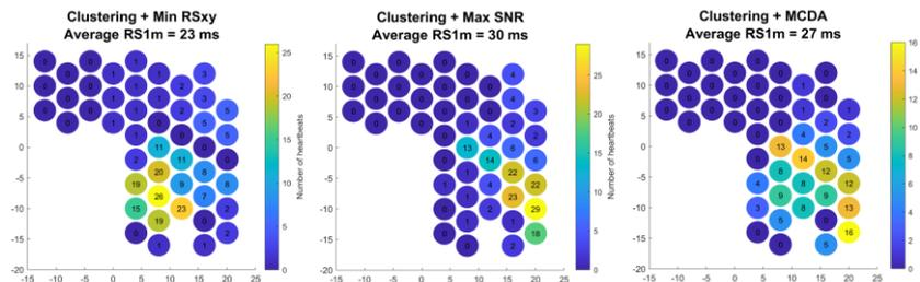
Number of times each microphone was selected using each tested approach for the identification of the best auscultation area (mitral valve).
