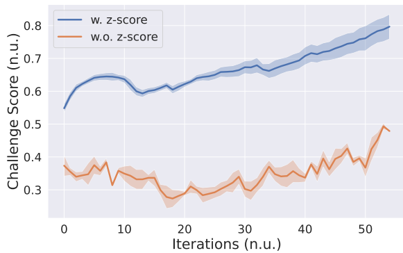
Figure 1: Comparison between mean curves of challenge scores from multiple experiments on the training set with (w.) and without (w.o.) z-score normalization. Shaded areas are error bounds (standard error of the mean).
