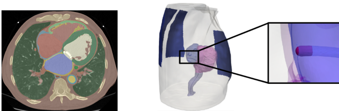
Figure 1: Left: CT scan image with different segments. Right: Torso geometry featuring an embedded catheter using Salome and a dispersive patch at various locations.
