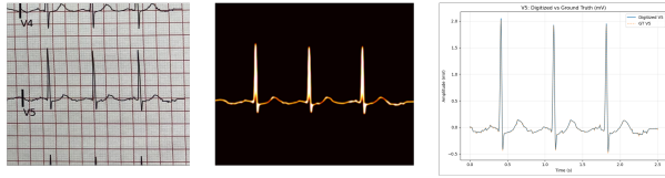
Figure 3: An example input (left), segmentation (middle), and digitised output (right) applying to the full pipeline. The SNR is 17.06 dB.
