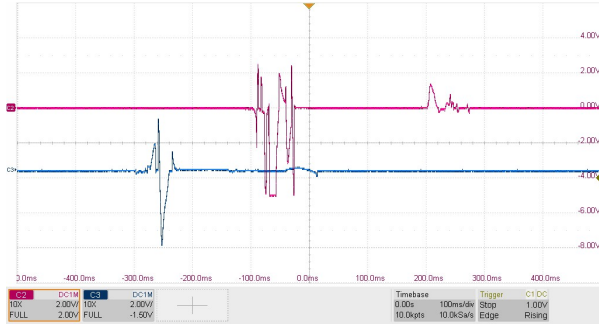
Figure 1. Oscilloscope trace of the 43-node PACER model with no external influence (pink trace correlates with VEGMs, and blue trace correlates with AEGMs).
