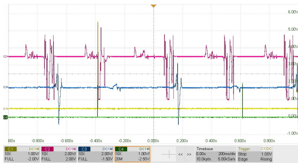
Figure 7. Oscilloscope trace of the 43-node PACER model pacing the right atrium with a voltage amplitude of 1.9 V.
