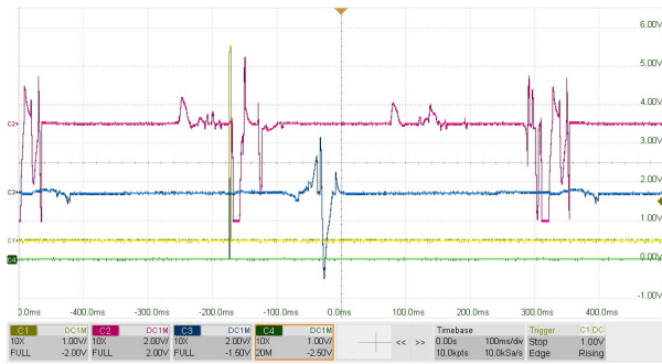
Figure 8. Oscilloscope traces of the 43-node PACER model pacing the right atrium with a voltage amplitude of 2.1 V.
