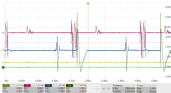
Figure 5. Oscilloscope traces of the 43-node PACER model pacing the right atrium with a voltage amplitude of 2.1 V.
