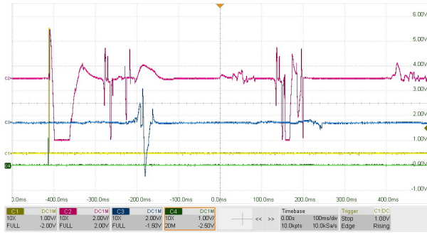
Figure 6. Oscilloscope traces of the 43-node PACER model pacing the right ventricle with a voltage amplitude of 1.1 V.
