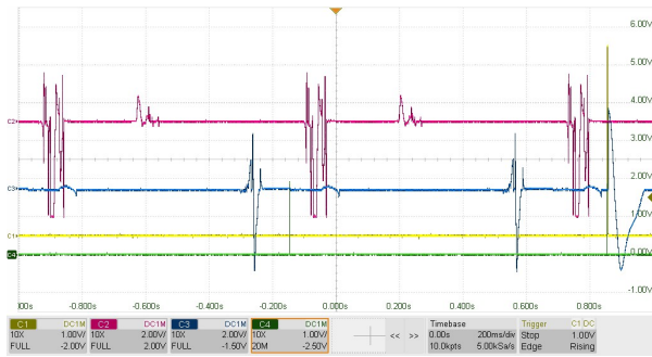
Figure 4. Oscilloscope traces of the 43-node PACER model pacing the right atrium with a voltage amplitude of 1.9 V
