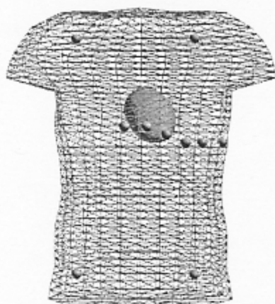
Figure 1. Triangulated torso geometry, location of canine ventricles, and location of 12 lead ECG electrodes.
