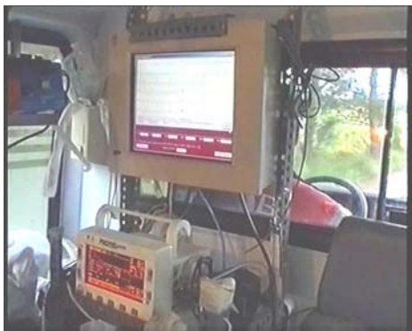
Figure 5. The internal setting of the ambulance with the panel PC and the vital sign monitoring.
