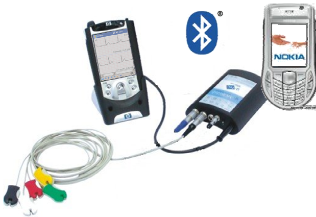
Figure 3. Data acquisition and transmission equipment. ECG signals are recorded with a mobile biosignal acquisition system (g.mobilab, g.tec – Guger Technologies OEG) that is connected with a PDA. A mobile phone is used for sending the ECG to the telemedicine service centre.
