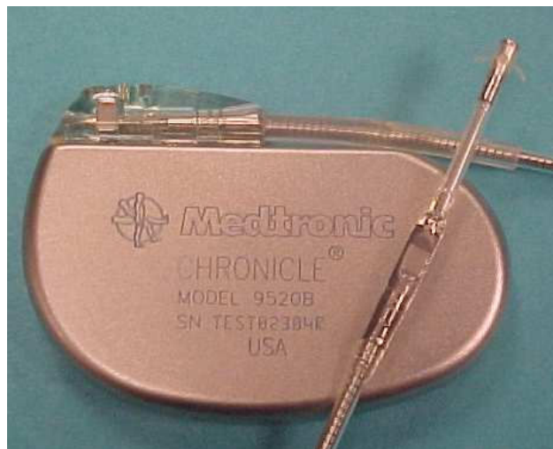
Figure 1: Chronicle® implantable hemodynamic monitor (Medtronic Inc.) The system consists of a memory device, a pressure lead and an external pressure reference.
