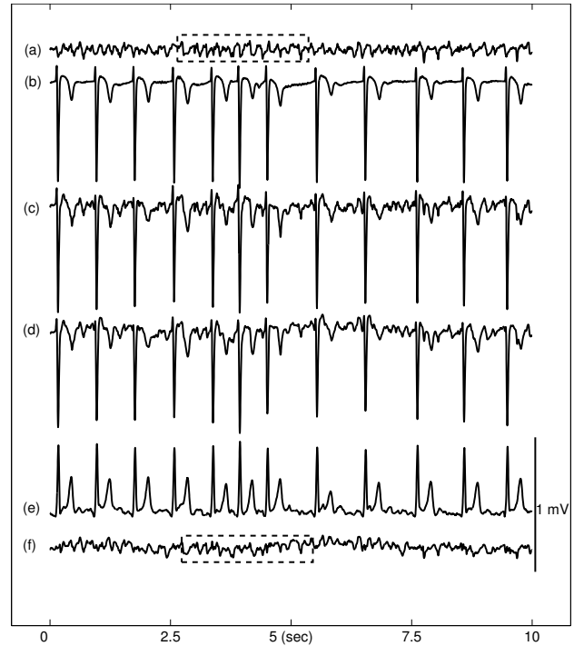
Figure 2. (a) Original 10-second ECG signal on V1. (b) Real VA on V1 from a 78 years old patient in sinus rhythm (c) Sum of the AA and VA on V1. (d) Baseline correction on V1 (e) Total RMS signal after baseline correction. (f) Estimated AA with the proposed method. (Boxed-in segments are shown magnified in Figure 3)
