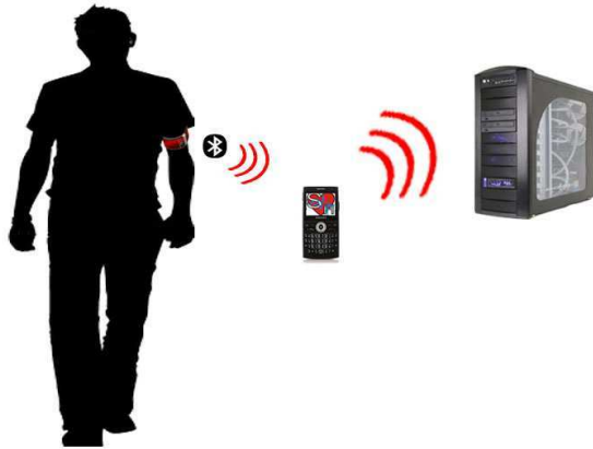
Figure 1. The block diagram of the autonomic computing system proposed. The system is compound of three parts: a cuff, a mobile device that controls the operation of the cuff and a server.
