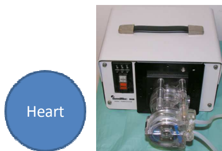
Figure 4. Roller pump (Ismatec BVP) representing the heart
