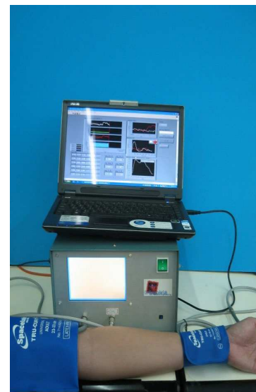
Figure 1. The continuous blood pressure measurement system.
