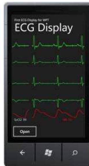
Figure 1: 4 Channel ECG and pulse wave on a Smartphone Emulator. Attention: ECG and pulse wave are form different simulators and therefore not synchronized.
