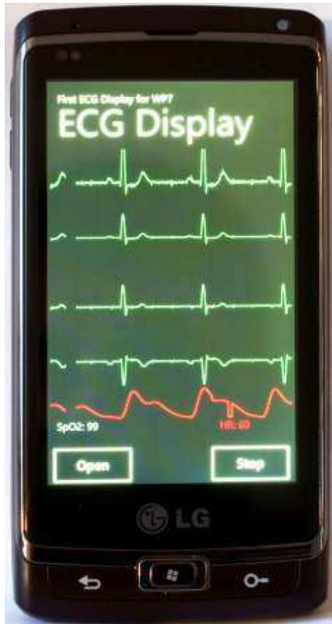
Figure 4: Application on a real Windows Phone 7. 3.5” touchscreen Resolution 480-by-800 pixels. The approximate size of the smartphone is : 116 x 59 x 16 mm. Attention: ECG and pulse wave are form different simulators and therefore not synchronized.
