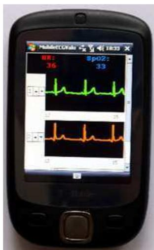
Figure 5: A biomedical ECG viewer shown on an old Windows Mobile 6.0 device with a 2.8” touchscreen and a screen resolution of 240-by-320 pixels [4].
