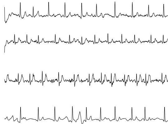
Figure 1. Four signals annotated as normal sinus rhythm which the algorithm places in the high priority group due to an irregular beat pattern which cannot be explained by quality issues, SVES/bigemini behavior or other ectopic beats. The ten first seconds out of 30 are shown.
