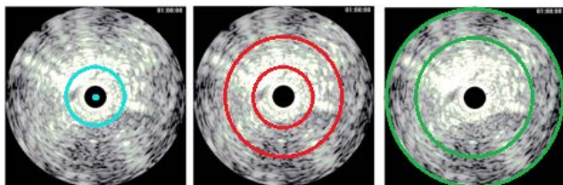
Figure 1. Logarithm of a RF image with div=3 and from left to right: k=3 (region of the catheter), k=2 (middle ring) and k=1 (border ring). Selecting the set (div=3,k=2), the ROI used for the correlation would be the middle ring.
