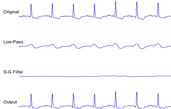
Fig. 8. Performance of SG baseline filter on an ECG without baseline. Duration is 4s and R-wave peak amplitude is 0.2mV.
