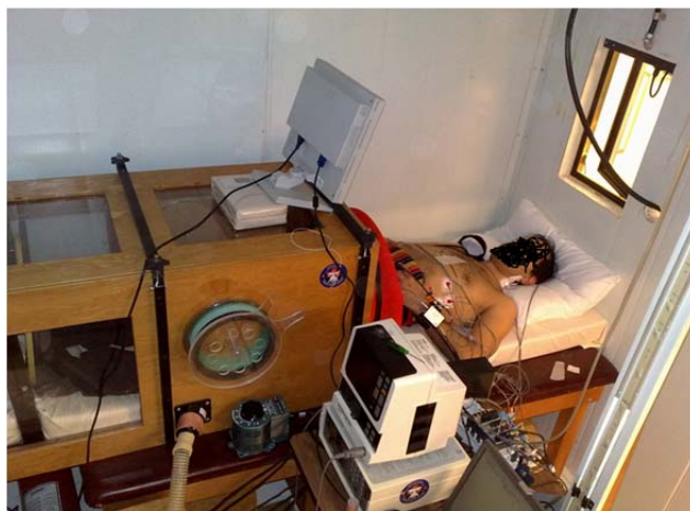
Figure 1. The LBNP and data acquisition setup. A vacuum was used to reduce the pressure inside the chamber. SCG, ECG and blood pressure were recorded simultaneously. Echocardiogram was also used for 18 participants to measure cardiac output and stroke volume.
