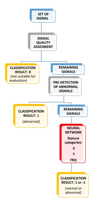
Fig.1 Flow chart of PCG classification algorithm.
