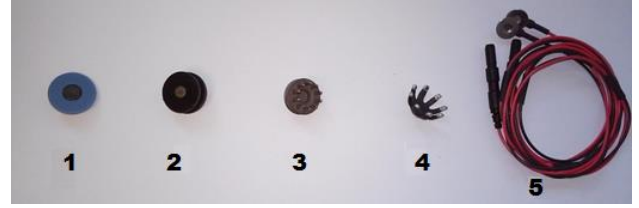
Figure 4. Dry electrodes used for the measurements.
