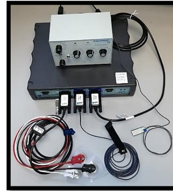
Figure 2: ECG sensor (Left), PPG Sensor (Center), BPP sensor (right), Biopac MP36R (bottom) and Film Lab amplifier (top)
