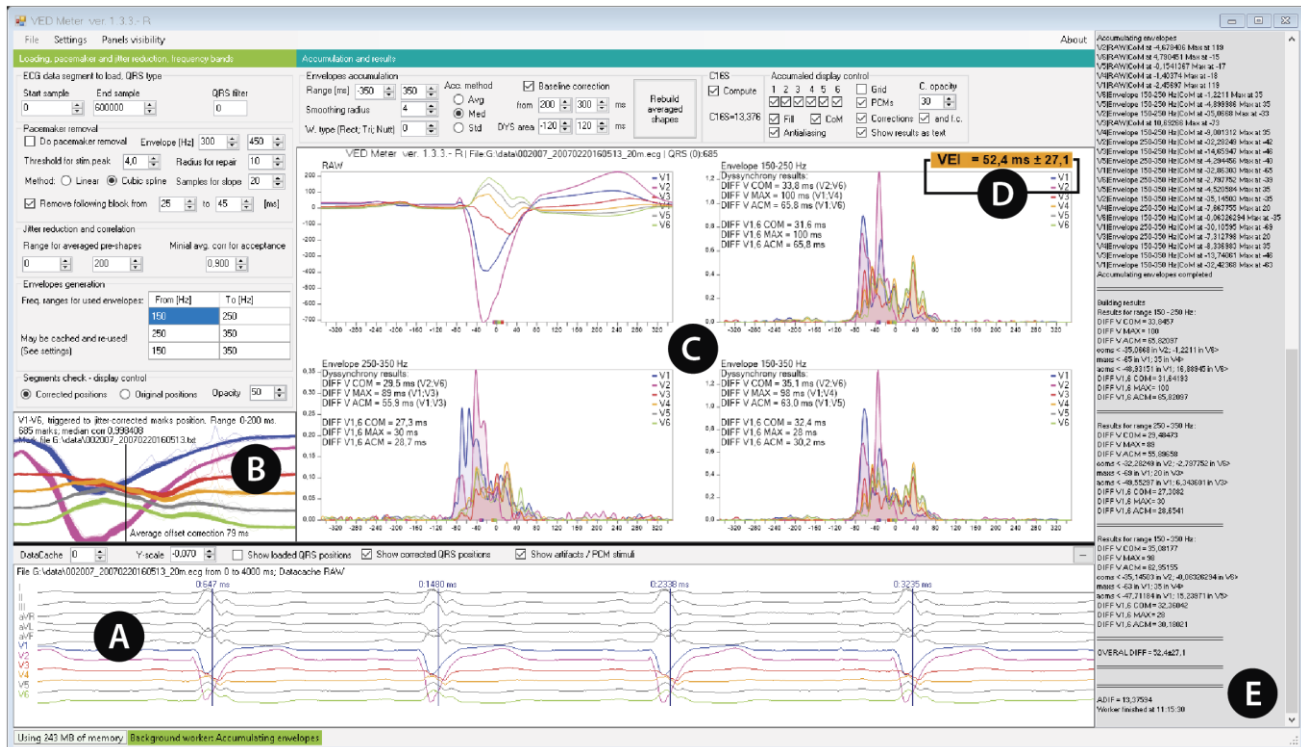
Figure 3: VED Meter – GUI and results display. Interactive preview of input signal (A), panel allowing check of jitter removal (B), display of averaged QRS, median shapes and intermediate results (C) and the VED value (D). Additional computing info is displayed in the right panel (E).
