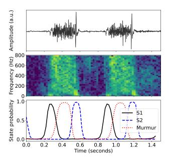
Figure 1. Generation of neural network state predictions for a murmur signal. A phonocardiogram (top) is transformed to a normalised spectrogram (middle) that is input into an RNN that predicts heart sound states (bottom).
