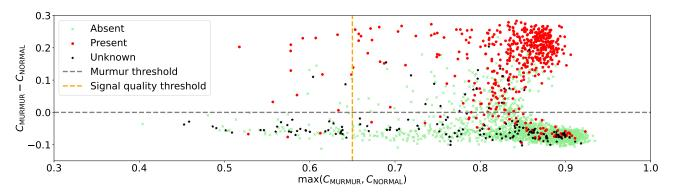
Figure 2. Confidences in the murmur ( $C_{MURMUR} = max(C_2, C_3, C_4)$ ) and normal ( $C_{NORMAL} = C_1$ ) segmentations are used to predict murmur likelihood ( $C_{MURMUR} - C_{NORMAL}$ ) and a signal quality metric ( $max(C_{MURMUR}, C_{NORMAL})$ ), which are plotted here for every signal in the training set. The marker type indicates the ground truth label. The dashed lines show the thresholds which then partition the points into 'Murmur Present', 'Murmur Absent' and 'Unknown' predictions.
