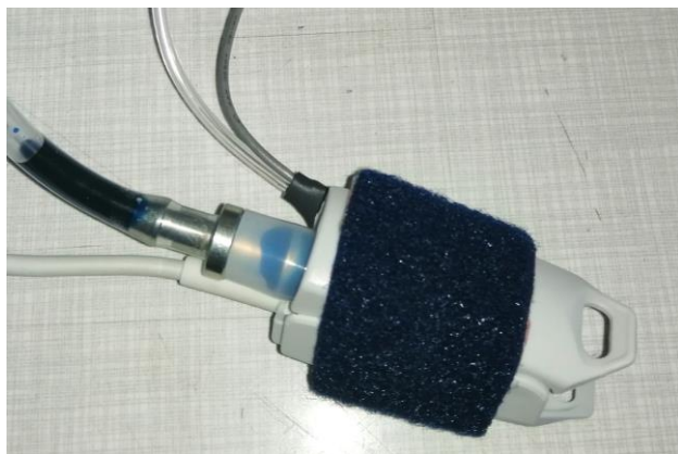
Figure 2. Photography of the silicon phantom with attached photoplethysmography sonde and pressure cuff. Silicon cylinder was filed with dark blue water.
