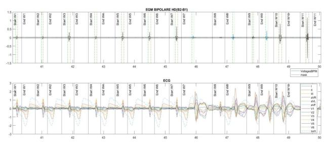
Figure 4 Ventricular EGM with the start of a VT, green (start) and red (end) dashed lines identifying the activations on the EGM. Black vertical lines are the corresponding search windows from the ECG.
