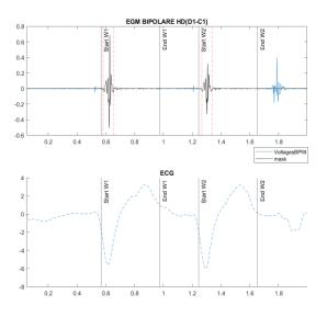
Figure 2 EGM and ECG signals showing both the windowing (black vertical lines) and the estimated duration (dashed red lines) of the algorithm.
