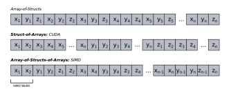
Figure 1. Different data layout representation, in Arrayof-Structs-of-Arrays (AoSoA), each component is stored in smaller contiguous chunks corresponding to the size of the vector extension. In SoA, the large contiguous chunks of memory for each variable have benefit in terms of contiguous memory accesses for CUDA kernels
