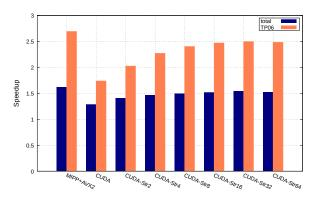
Figure 3. Comparison of the speedup for model M on 2 MPI nodes (64 OpenMP threads in total) on Broadwell architecture.
