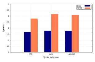
Figure 5. Comparison of the speedup of vectorization according to Vector Extensions for model M on 2 MPI nodes (72 threads) on Cascade Lake architecture.
