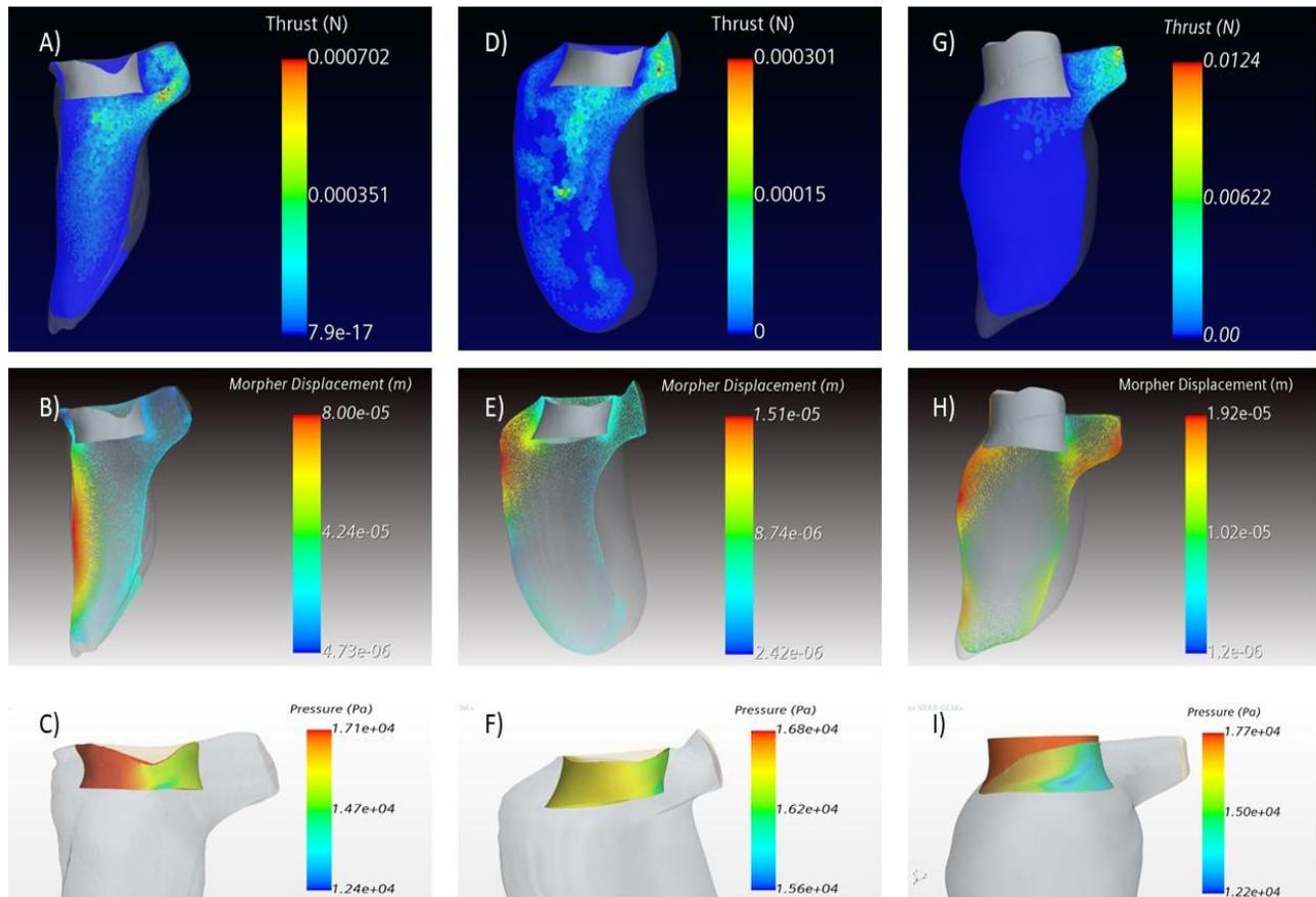
Figure 1 -visualisation of thrust, morpher displacement and pressure fields for VIM-1 (A-C), VIM-2 (D-F) and VIM-3 (G-I)
